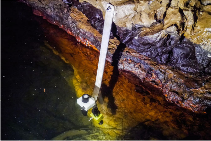
Fig. 4.2 Observation point with instrument with programmable data logger ( Photo M. Blatnik )
